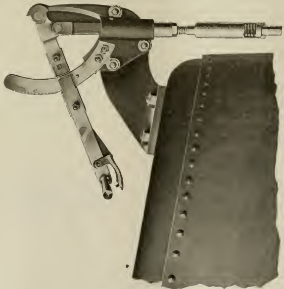
CHAMBERS THROTTLE RIGGING IN LOCOMOTIVE CAB.
